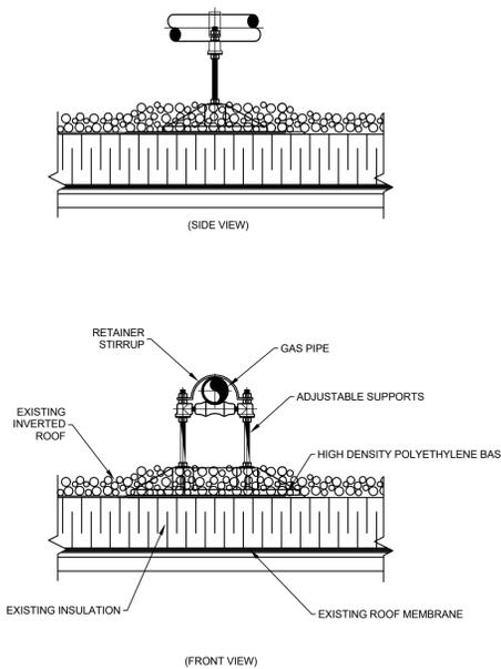
**GAS PIPE SUPPORT ON FLAT ROOF DETAIL**
